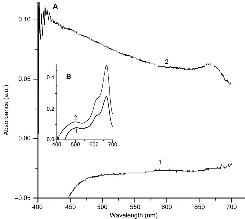
Fig. 5. Absorption spectra of culture samples: 1 – acetate culture; 2 – lactate culture after 2 days of cultivation (A) and 17 days (lactate culture) or 32 days (acetate culture) of cultivation (B) with methylene blue method's reagents.
