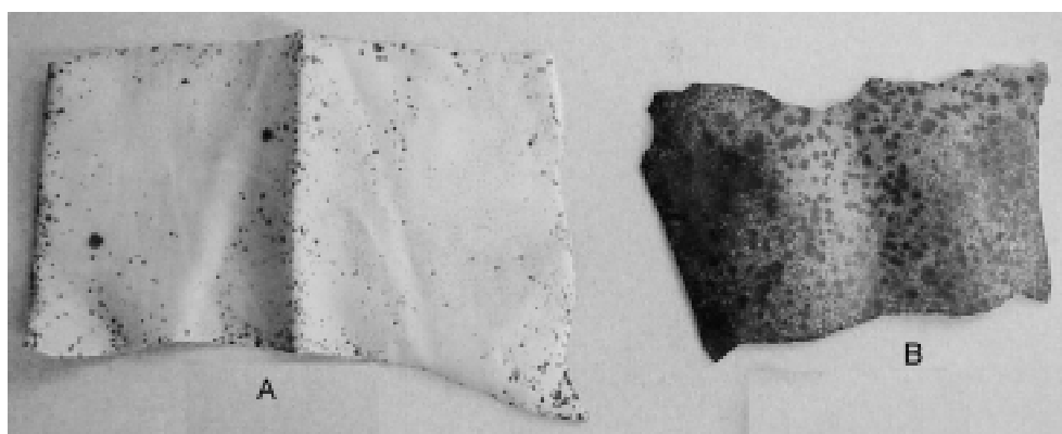
Fig. 2. Enhanced degradation of NR-latex gloves by Achromobacter sp. NRB. A nontreated, B treated.
