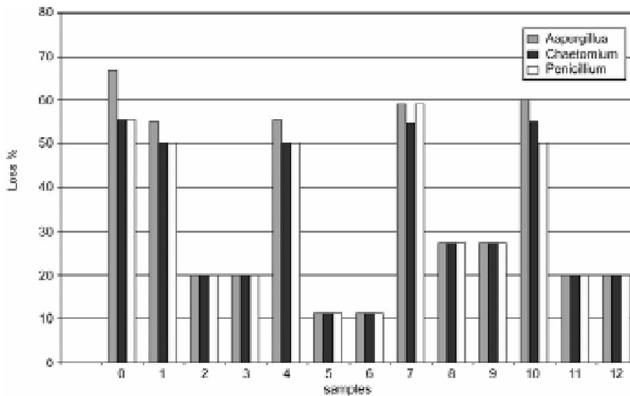
Fig. 2. The loss % in the elongation of the sampes after the fungal treatment.
