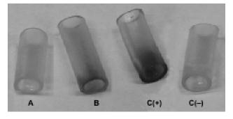
Fig. 2. Image of infusion tube colonized by *S. aureus* biofilm: A, B – treated for 24 h with TTO, respectively at MIC or ½ MIC. C(+) – not treated positive control, C(–) – not colonized negative control. TTC-reduction assay – scored according to an arbitrarily fixed scale as described in Material and Methods.
